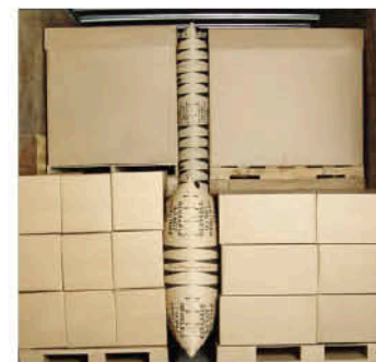
Positioning of the Dunnage Bag
