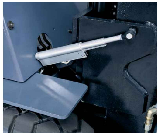
Tilt indicator mounted between cowl and mast.
