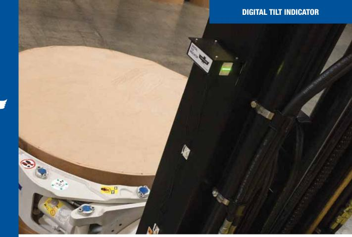
Reduce load damage by always picking up the load at true vertical.
