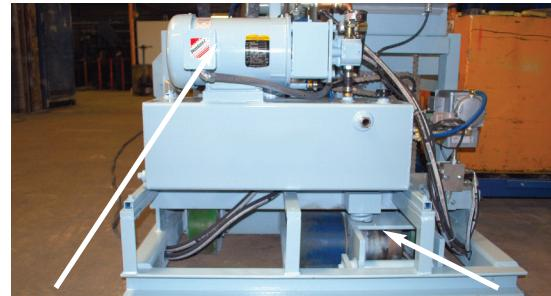
Hydraulic Power Unit      Drive Motor and Wheel
