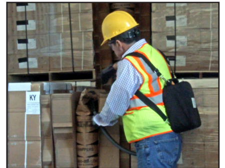
Fill airbags as you go – easy to get into and out of trailers
