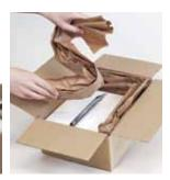
The converter forms single layer kraft paper into a high volume star-shaped paper configuration, which can be used as an effective filling material. It prevents products from shifting around in their box, ensuring damage-free arrival at the end destination. The converted paper gets dispensed directly at the point of operation, improving the efficiency of the packaging process and optimizing the speed of working.
