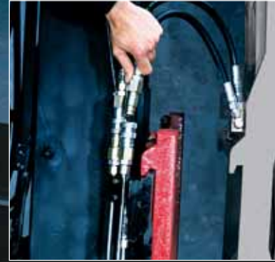
3. Connect hydraulic lines
