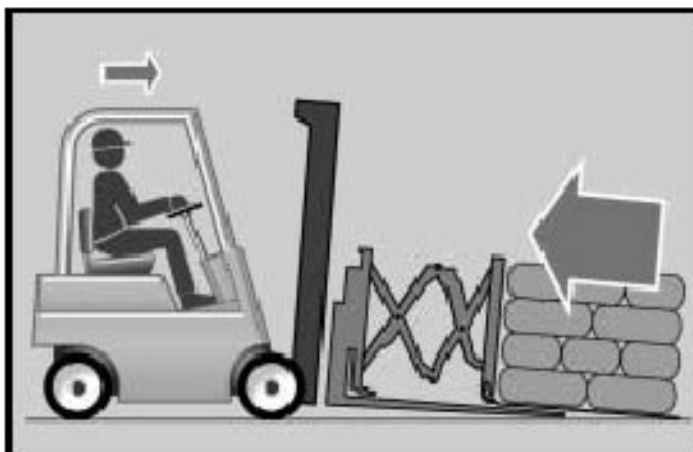
3. Move forward slowly as the load is being pulled onto the platens.
